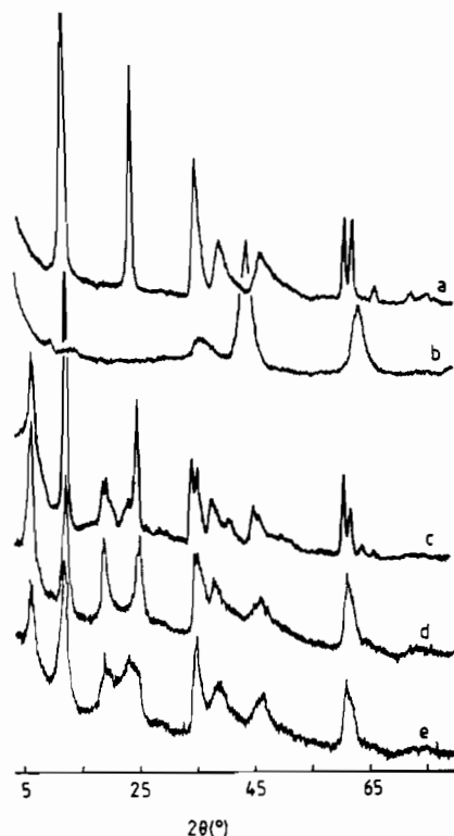
Figure 1. Powder X-ray diffraction patterns for (a) MGALCO 3 , (b) MGALCAL550, (c) MGALT1, (d) MGALT2, and (e) MGALT2G.
